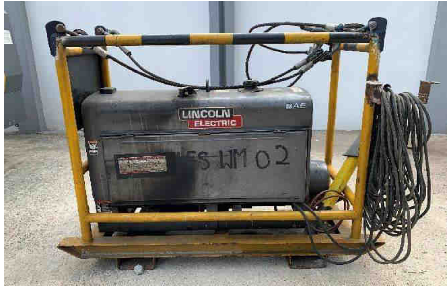
Lincoln Welding Machine - SAE 300Amps
