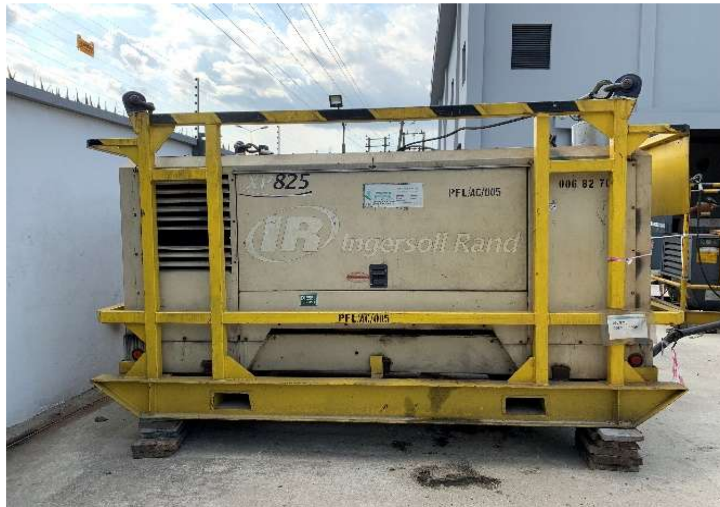
Ingersoll Rand 900CFM Compressor
