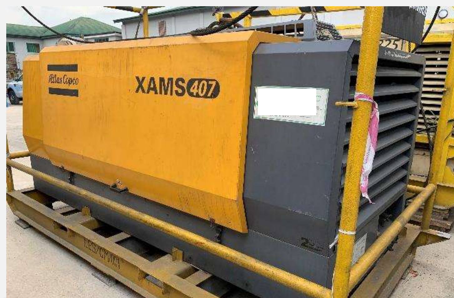
Atlas Copco - 900CFM Compressor
