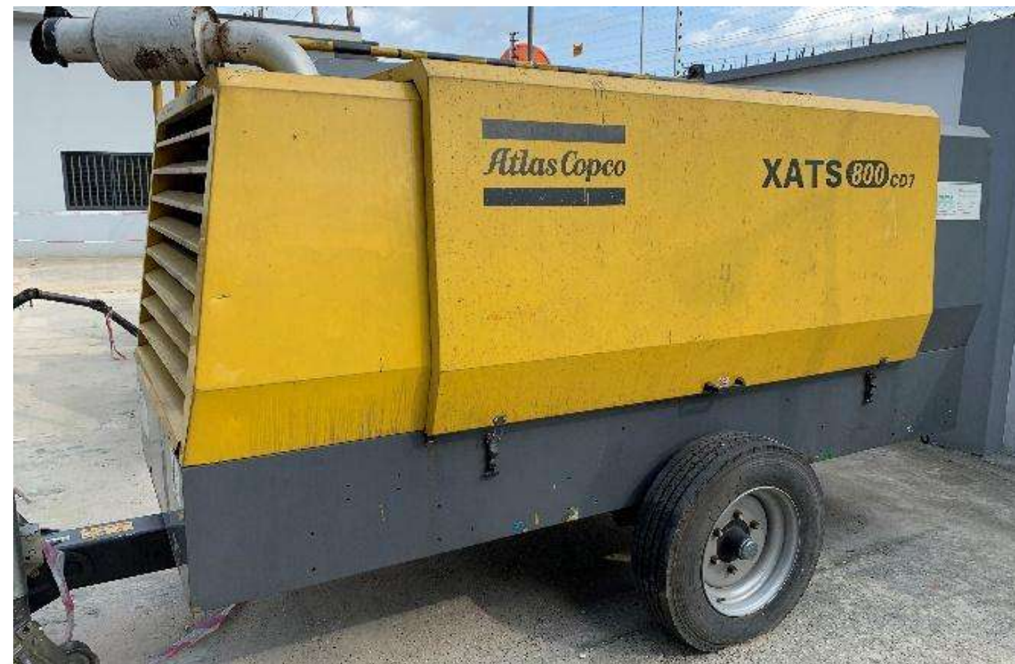
Atlas Copco - 900CFM Compressor
