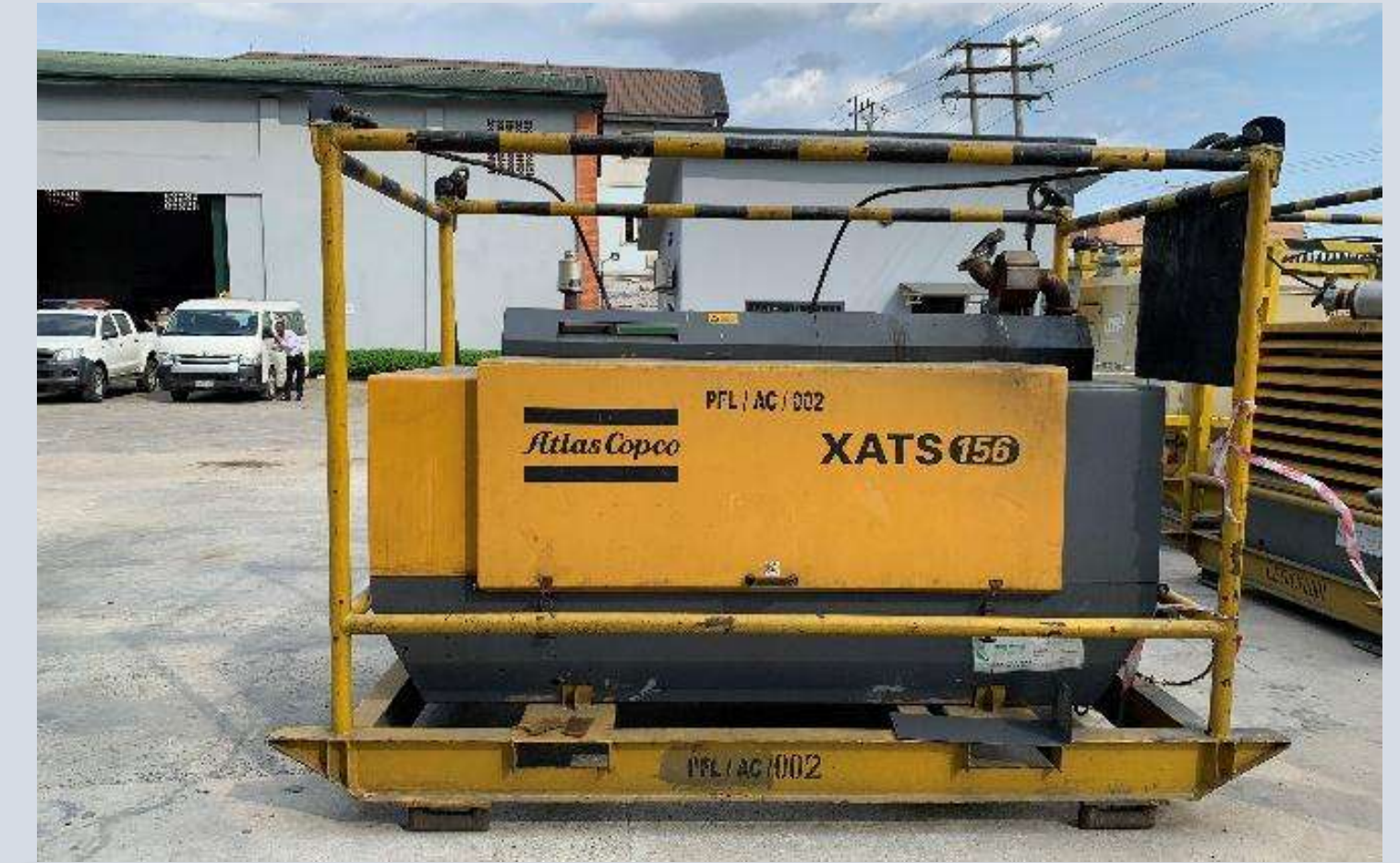
Atlas Copco - 400CFM Compressor
